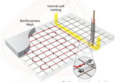
Flexible conduit tied to mesh with heating cable into room
